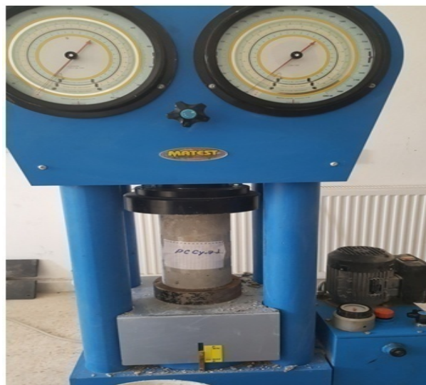
Figure 3. Testing cylindrical specimen.
