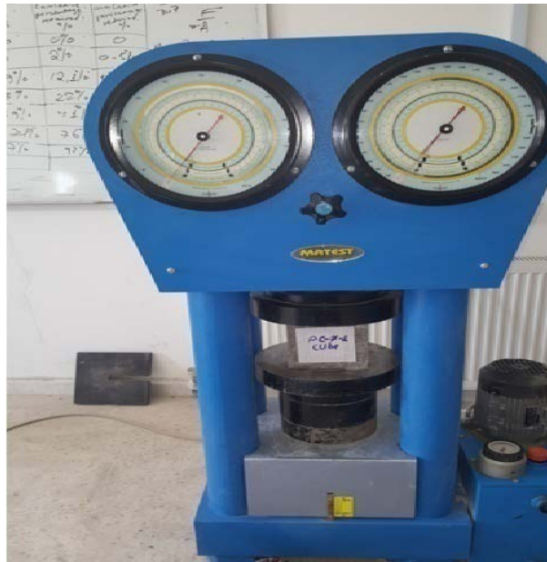
Figure 2. Testing cube specimen.
