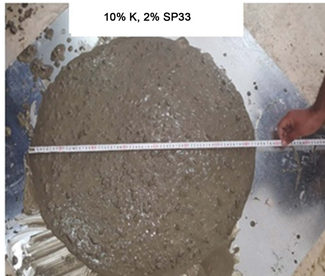
Figure 4. SCC mix with 10% K + 2% SP33.
