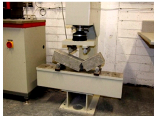
Fig. 3. Testing of beam specimens in flexure.
