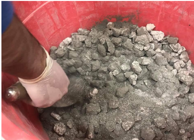
Fig.(8). Dry mixing
