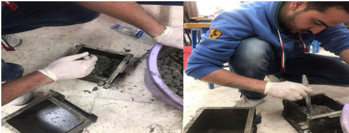
Fig.(10).The process of compacting
