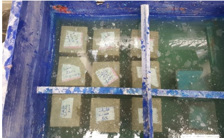
Fig.(12). Cubes Curing (Water Treatment)
