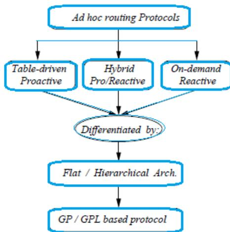
Fig. 1 Classification of ad hoc routing protocols
