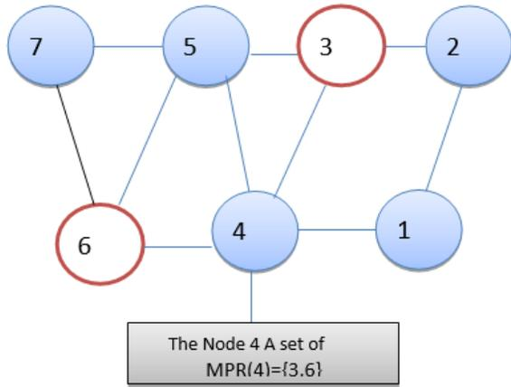
Fig. 2 fragment of a distributed radio network
