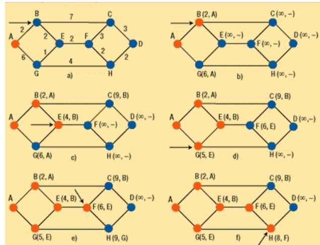
Fig. 6 The definition of the shortest path
